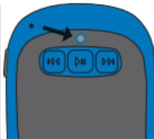
**NOTE:** When unit is fully charged, indicator light will be solid BLUE.
